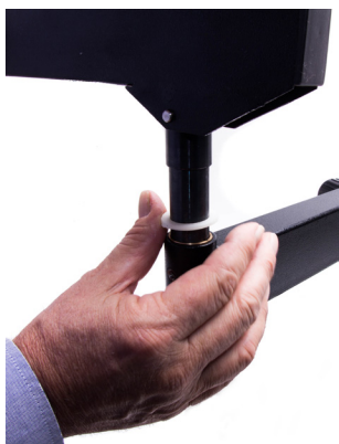
Fig. 7—(Left) Slide the post of the adjustable forearm into the hole on the middle horizontal bar.
