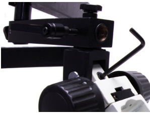
Fig. 22—Adjust the tension on the focus mount hinge using the hex key provided with the 502009 focus mount.
