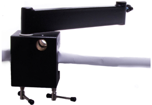
Fig. 4—(Left) Line up a ring washer with the hole on the table clamp.
