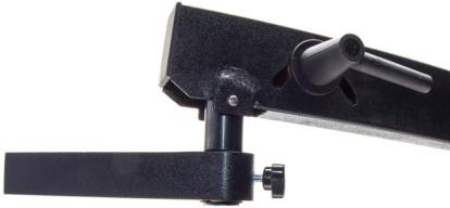
Fig. 9—Install an adjustment screw in the small horizontal bar.
