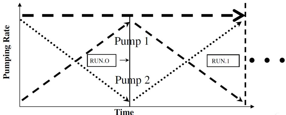
Maintains a constant total flow rate between 2 syringe pumps. A gradient (Linear function) dispensing function is programmed into the Master pump. The secondary pump will be automatically programmed with the inverse of the Master pump's gradient function. The sum of the two pump's flow rates will be a constant. Both pumps will increase and decrease pumping rates in tandem.
