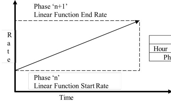
The Linear Flow Rate function is specified by using two Linear Functions **LInr**, in two consecutive Program Phases, defined by four parameters:
