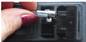
Fig. 28—Open the fuse housing and rotate it right to remove the fuse.
