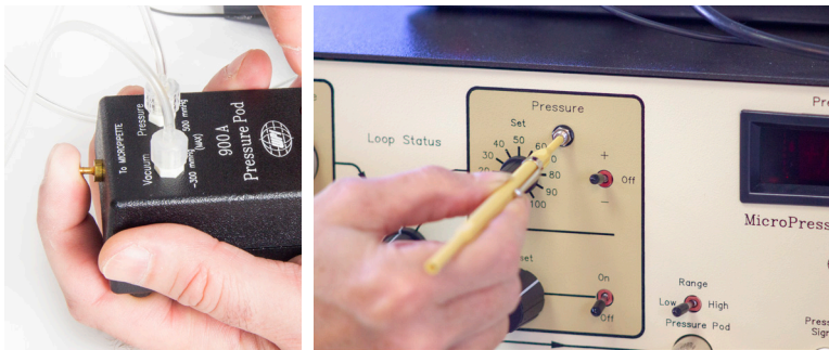
Fig. 7—Use your finger to block the To Micropipette port on the top of the Pressure Pod. Fig. 8—Use a screwdriver to adjust the recessed Pressure screw until the meter reads zero.
