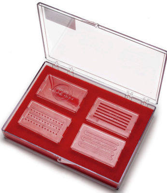
Fig. 4—Z-MOLDS come in four different patterns. Press into freshly poured agarose and allow the agarose to solidify. Remove the mold. The impressions make it easy to hold embryos.
