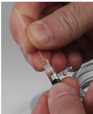
Fig. 13—Press the glass micropipette into the electrode holder.
