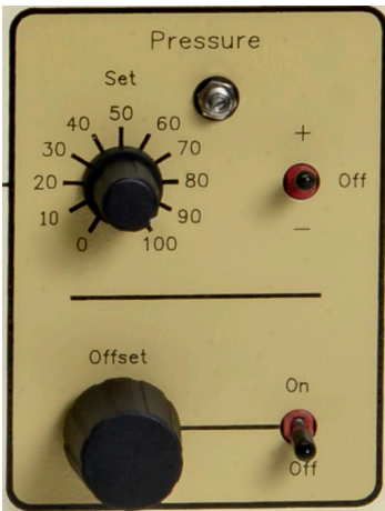
Fig. 21—Turn on the pressure offset and use the dial to bring the 900A display to zero.
