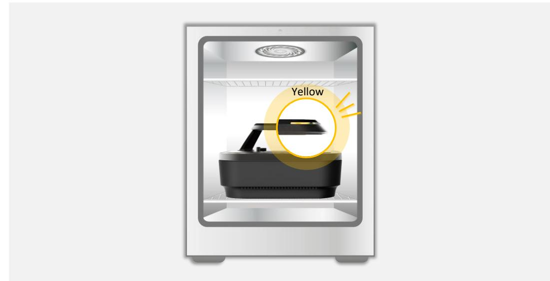
**Step 1.** Place the sample on the stage of the Celloger® Pro. Make sure the A1 of the plate and stage are aligned.
