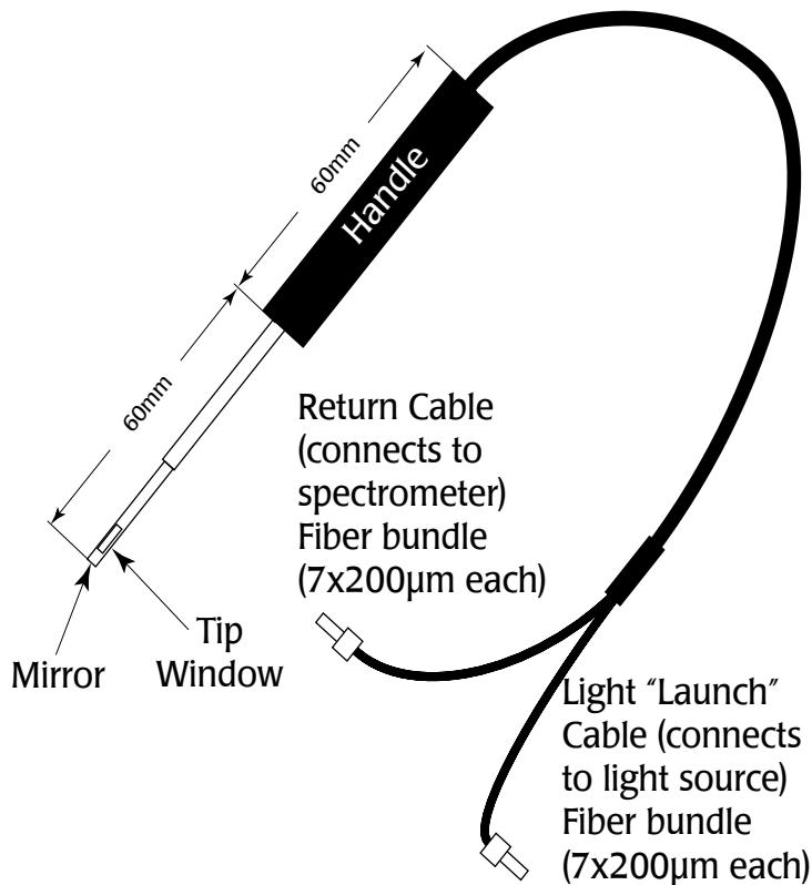
Connect the fiber optic connectors to the spectrometer and the light source. Hold the Mini DipTip by the handle. Don't bend the tip.
