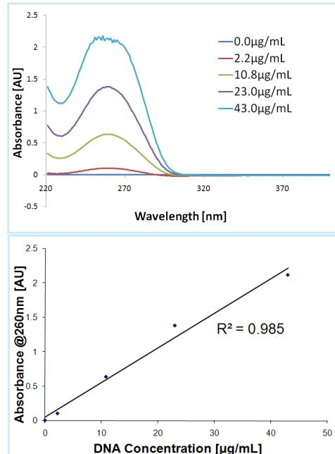
DNA samples (with a sample volume of 50µL inside mini centrifuge PCR vials) were measured in PBS with concentrations 0-43µg/mL using a Tidas 100 spectrophotometer.
