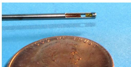
*This tiny shaft contains 14 fused silica fibers, all polished to a perfect tip. Light travels through seven fibers through the sample. It is reflected off a mirror in the tip and returns to the spectrometer through the sample and the other seven fibers.*
