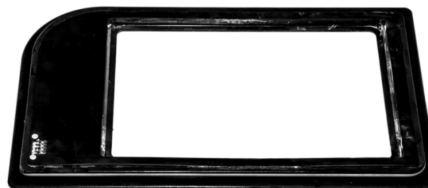
Fig. 23—The rounded corner of the lid fits into the thumb hold on the base of STEV. Notice the electronic interface connection in the bottom left corner of the image. This interface allows the controller to communicate with the lid and control the lid temperature.
