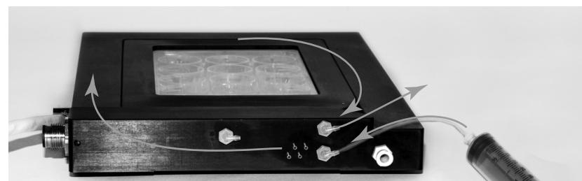
Fig. 4—Use a large syringe filled with distilled water to fill the water reservoir. When it is full, water will come out the overflow port.
