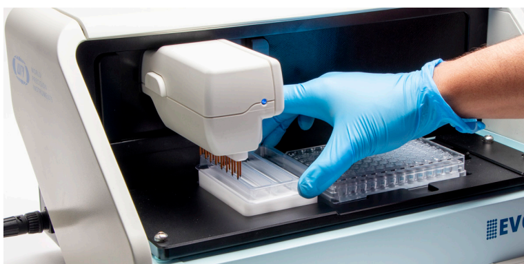
Fig. 6—Place a sterile disposable rinse station insert in the base rinse station. Discard it and use a fresh rinse station insert before installing a different plate or running a different set of experiments
