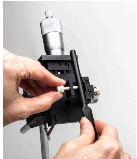
Fig. 7—(Left) The electrode should be positioned in the groove in the bracket.
