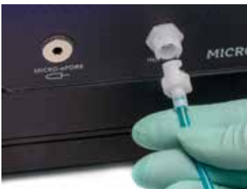
Fig. 12—(Left) Align the connector with the Injection Port, slide the connector in position and rotate the connector a little clockwise to lock it into place.
