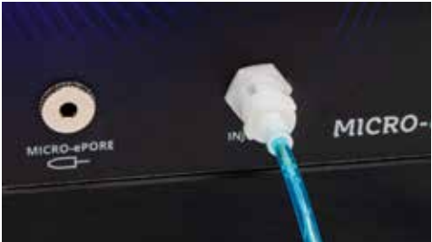
Fig. 12—(Left) Align the connector with the Injection Port, slide the connector in position and rotate the connector a little clockwise to lock it into place.
