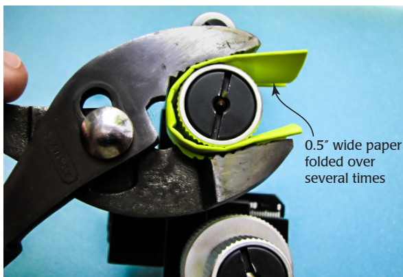
Fig. 5—Wrap the knob with a thick layer of papers so the pliers do not gouge the aluminum knob.
