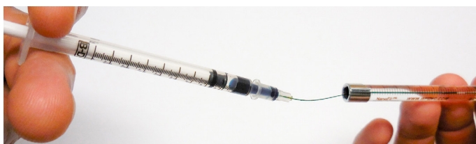
Fig. 7—Pre-load method of syringe filling.
