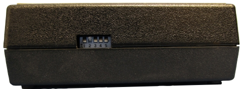
Fig. 3 —The right side of the controller box has five DIP switches for controlling aliquot injection volumes and injection speeds
