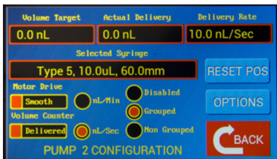
Fig. 19—The Configuration screen allows you to set the limits of travel and define parameters for a selected pump.
