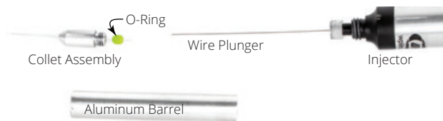
Fig. 13—(Left) The injector is disassembled to replace the gaskets.
