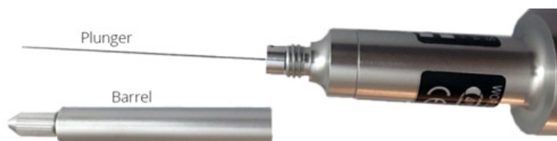
Fig. 46—The barrel is removed to expose the plunger.
