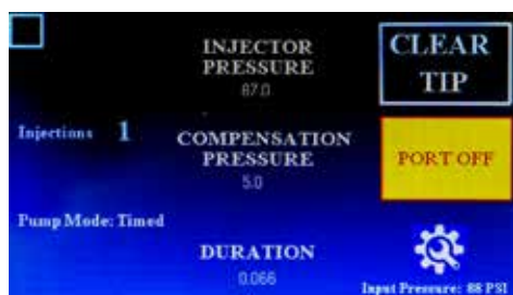
Fig. 10—The warning indicates that the injection port is disabled by default on startup. To enable the port, press the Port OFF button. The Port OFF message will become the Inject button.
