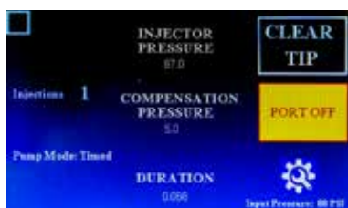
Fig. 25—When the Injection Port is disabled a notice appears on the main screen.
