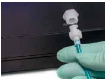
Fig. 12—(Left) Align the connector with the Injection Port, slide the connector in position and rotate the connector a little clockwise to lock it into place.
