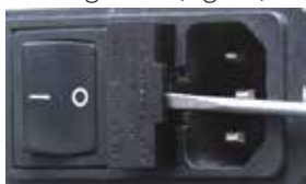
Fig. 16—Insert the screw driver under the fuse housing lip and pry the housing open.
