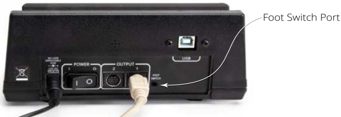
Fig. 2—The port for the footswitch is located on the rear panel of the MICRO2T controller.
