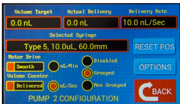
Fig. 35—Use the Configuration screen to enter all the parameters and select a syringe type.
