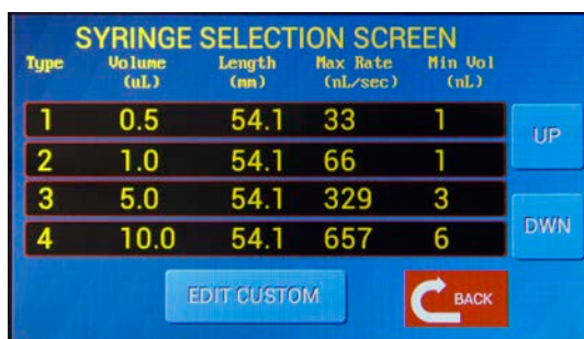
Fig. 14—The Syringe Selection screen allows you to choose from 10 default syringes and 3 user-defined syringes.
