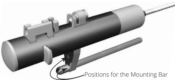
Fig. 10—Unscrew the mounting rod to reposition it.
