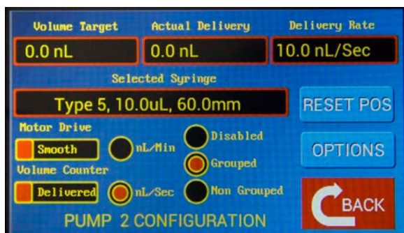
Fig. 26—The Configuration display shows the selected syringe type (Type 5) in the center of the screen.
