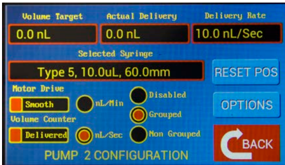
Fig. 16—The Configuration screen allows you to set the limits of travel and define parameters for a selected pump.
