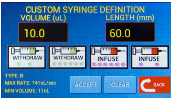
Fig. 28—Use the Custom Syringe Definition screen to define your new syringe type.
