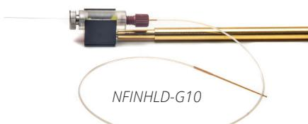
Use with the **NANOFIL** syringe and 1mm OD glass for your microinjection application."
