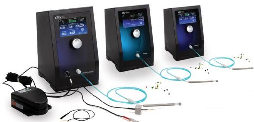
Designed to simplify intracellular injection and a variety of other microinjection tasks, WPI's **Microinjectors** use accurate timing and carefully regulated air pressures for securing cells and injecting. Injected volumes range from picoliters to nanoliters.
