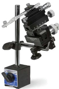
Weighing just 550 grams, the **M3301** is a well-built German micromanipulator that outsells all others worldwide for high precision experiments where magnification is in the range of up to 250x.
