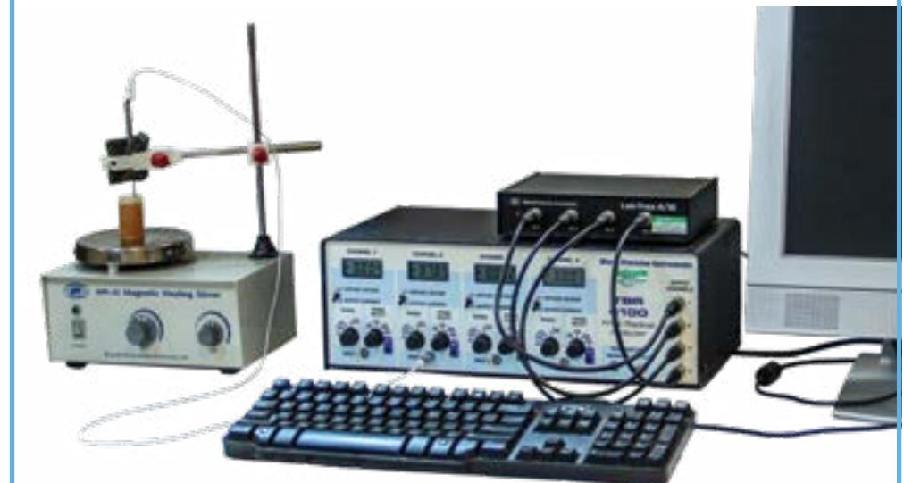
This is a typical laboratory setup of a WPI free radical analyzer with data acquisition system.
