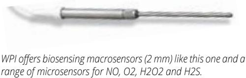
WPI offers biosensing macrosensors (2 mm) like this one and a range of microsensors for NO, O2, H2O2 and H2S.
