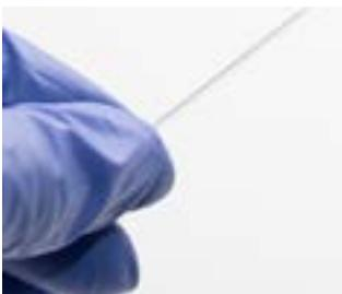
The pre-pulled glass pipettes (**UTips**) save the cost and time of making your own micropipettes.
