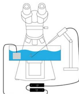
**CAUTION:** In applications where higher impedance microelectrodes, typically above  $2\text{ M}\Omega$ , will be immersed more than 4 or 5 mm into a conductive medium, additional insulation should be considered to minimize shunting. Polyimide tubing, which is used in our PT electrode models, is recommended.
