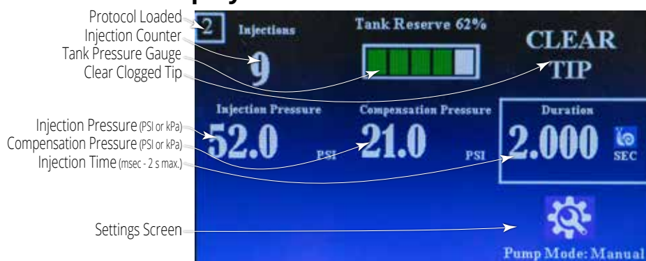
Fig. 4—The Touch Panel Display gives you access to all the parameters and the settings menu.
