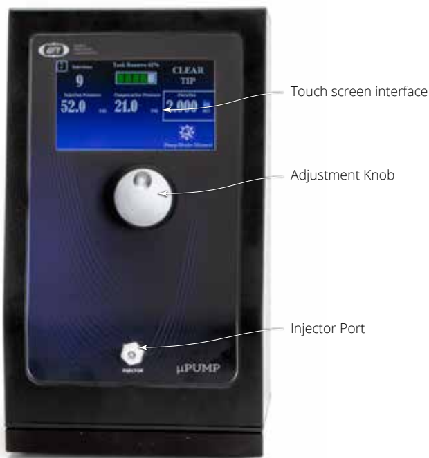
Fig. 2—The major features of the μPUMP are labeled in this diagram.
