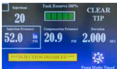
Fig. 24—When the Injection Port is disabled a notice appears on the main screen.
