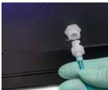
Fig. 11—(Left) Align the connector with the Injection Port, slide the connector in position and rotate the connector a little clockwise to lock it into place.
