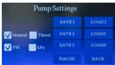
Fig. 23—The Settings menu lets you save enable or disable the Injection Port by pressing the Port ON/Port OFF toggle button.
