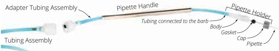
Fig. 10—The Capillary Kit must be properly assembled.
